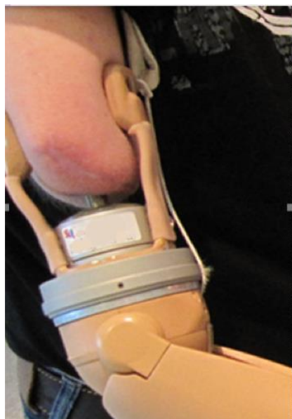
Figure 2: Osseointegrated prosthesis at transhumeral level with electrode holders. Foto courtesy of Carina Reinholdt.
