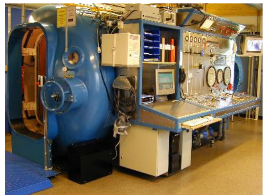
Traditional cylindrical hyperbaric chamber (SU/Eastern Hospital, Göteborg, Sweden)
