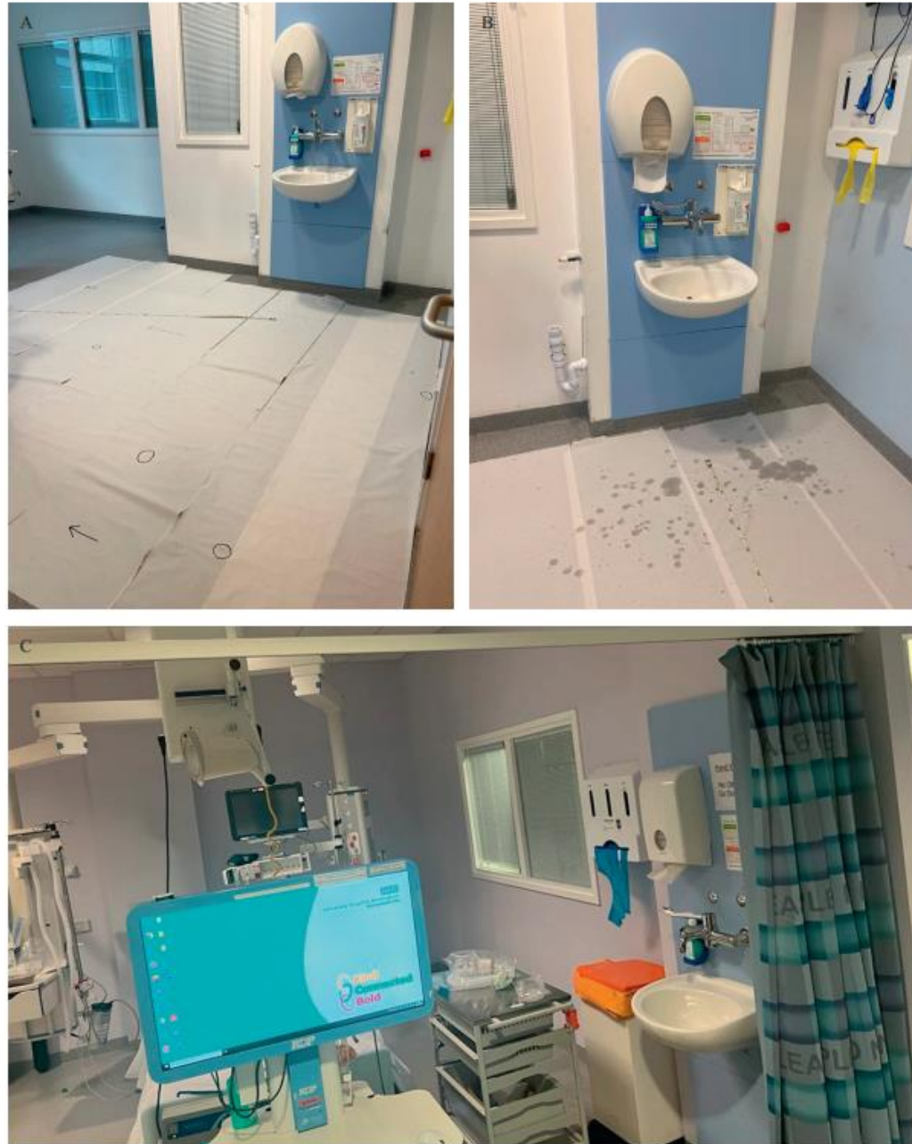
Figure 1. (A) Water from a running tap can splash some distance away from the sink, highlighted by circles on the paper towels on the floor. (B) Water can splash from undertaking hand hygiene, again highlighted by wet paper towels on the floor. (C) A typical intensive care unit patient bed space with equipment situated around a handwash basin.
