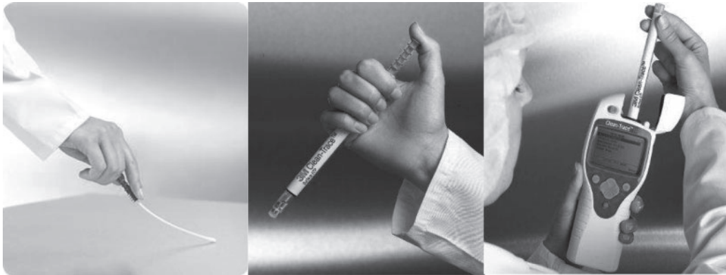
Fig. 2. Example of an ATP bioluminescence system. Note: Pictures of the 3M Clean-Trace system are used with permission from FOSS.
