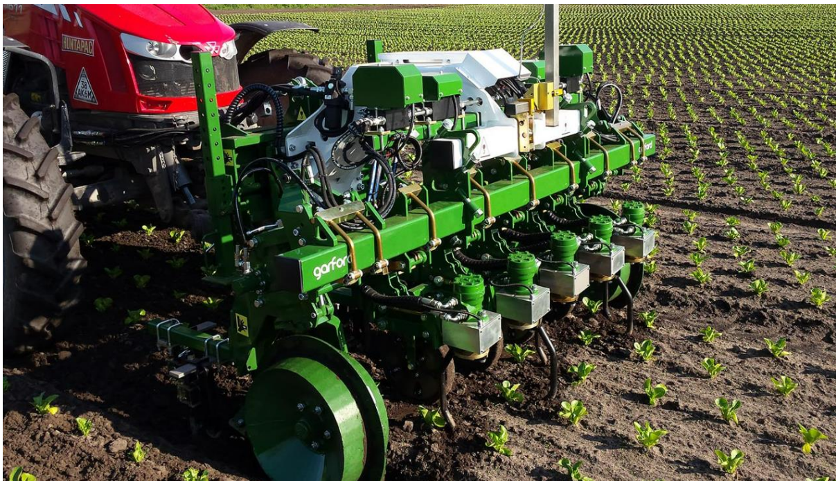
Figur 5. Kamerastyrd radhackning (Foto: Garford)
