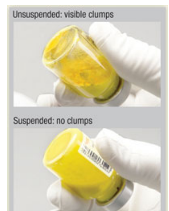
Figure 3: Check for unsuspended powder and repeat tapping if needed.
