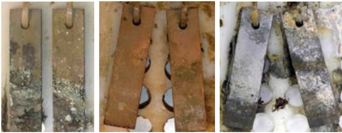
Figure 23. The brass coupons – above sediment recovered in 2004 after 2 years of storage (left), in 2005 after 1 year of storage (mid) and in 2009 after 5 months of storage (right).
