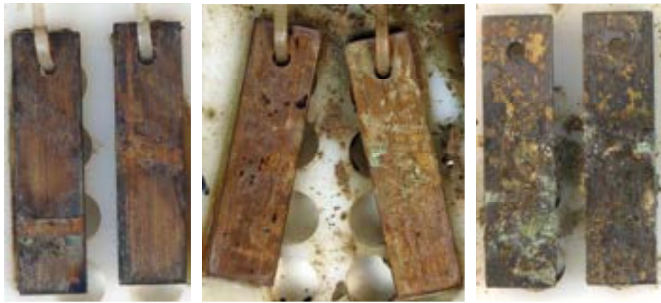
Figure 77. The brass coupons - 50cm below sediment recovered in 2004 after 2 years of storage (left), in 2005 after 1 year of storage (mid) and in 2009 after 5 months of storage (right).
