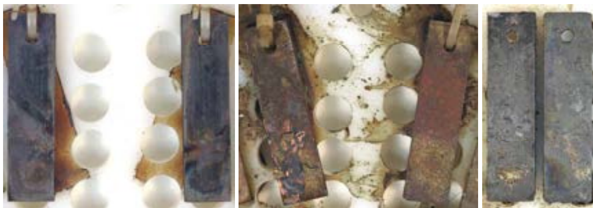
Figure 73. The copper coupons – 50cm below sediment recovered in 2004 after 2 years of storage (left), in 2005 after 1 year of storage (mid) and in 2009 after 5 months of storage (right).
