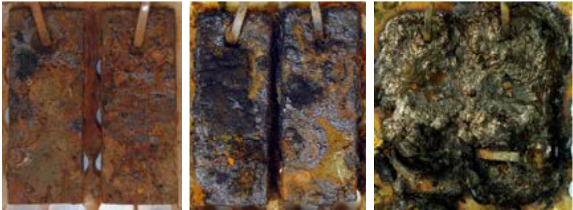
Figure 39. The cast iron coupons – above sediment recovered in 2004 after 2 years of storage (left), in 2005 after 1 year of storage (mid) and in 2009 after 5 months of storage (right).
