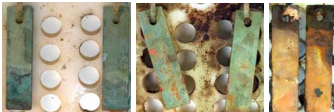
Figure 17. The copper coupons – above sediment recovered in 2004 after 2 years of storage (left), in 2005 after 1 year of storage (mid) and in 2009 after 5 months of storage (right).
