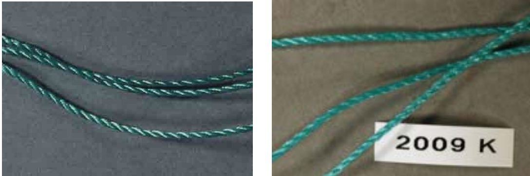
Figures 16 & 17. PE cord. Reference and samples retrieved after seven years of in-situ exposures in the sediments.
