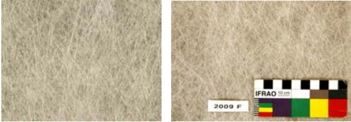
Figure 10 & 11. Geotextile of PP/PE. Reference and sample retrieved after seven years of in-situ exposures in the sediments.
