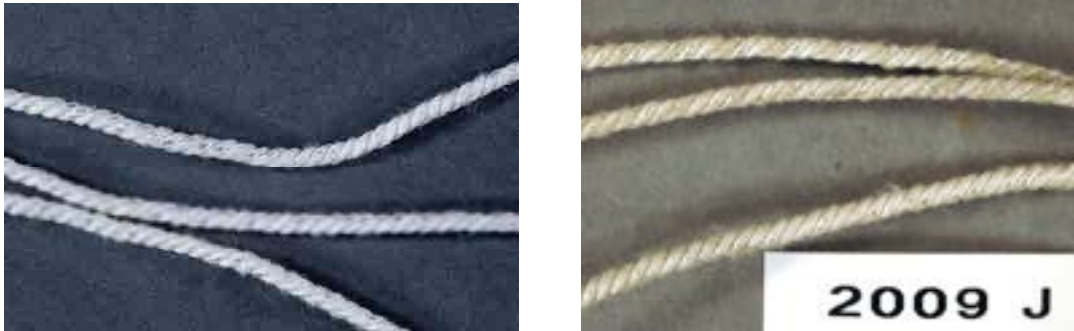
Figure13 & 14. Polyester cord. Reference and samples retrieved after seven years of in-situ exposures in the sediments.
