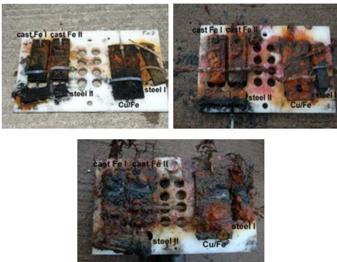
Figure 38. Ferrous alloy coupons – above sediment, immediately after recovery in 2004 after 1 year of exposure (top left), in 2005 after 2 years of exposure (top right) and in 2009 after 6 years of exposure (bottom).
