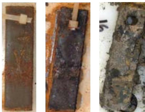
Figure 93. The mild steel coupons - 50cm below sediment recovered in 2004 after 2 years of storage (left), in 2005 after 1 year of storage (mid) and in 2009 after 5 months of storage (right).
