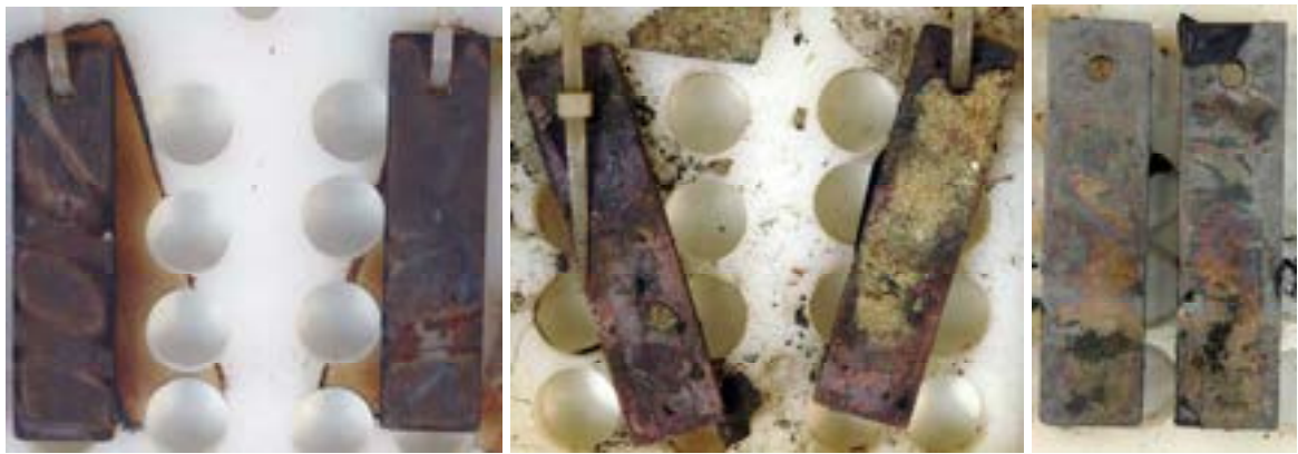
Figure 47. The copper coupons – just below sediment recovered in 2004 after 2 years of storage (left), in 2005 after 1 year of storage (mid) and in 2009 after 5 months of storage (right).
