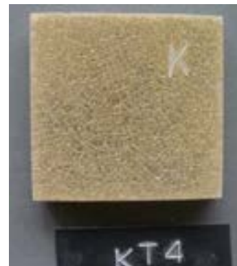
Figure 1b & c. Sample deposited in geotextile and retrieved after 7 years, in wet condition (b) and after drying (c)
