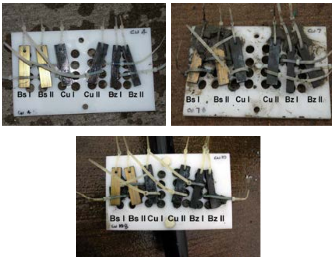
Figure 72. Copper alloy coupons – 50cm below sediment, immediately after recovery in 2004 after 1 year of exposure (top left), in 2005 after 2 years of exposure (top right) and in 2009 after 6 years of exposure (bottom).
