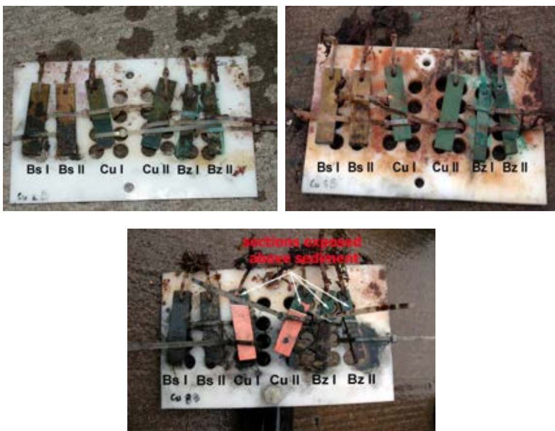
Figure 16. Copper alloy coupons – above sediment, immediately after recovery in 2004 after 1 year of exposure (top left), in 2005 after 2 years of exposure (top right) and in 2009 after 6 years of exposure (bottom).
