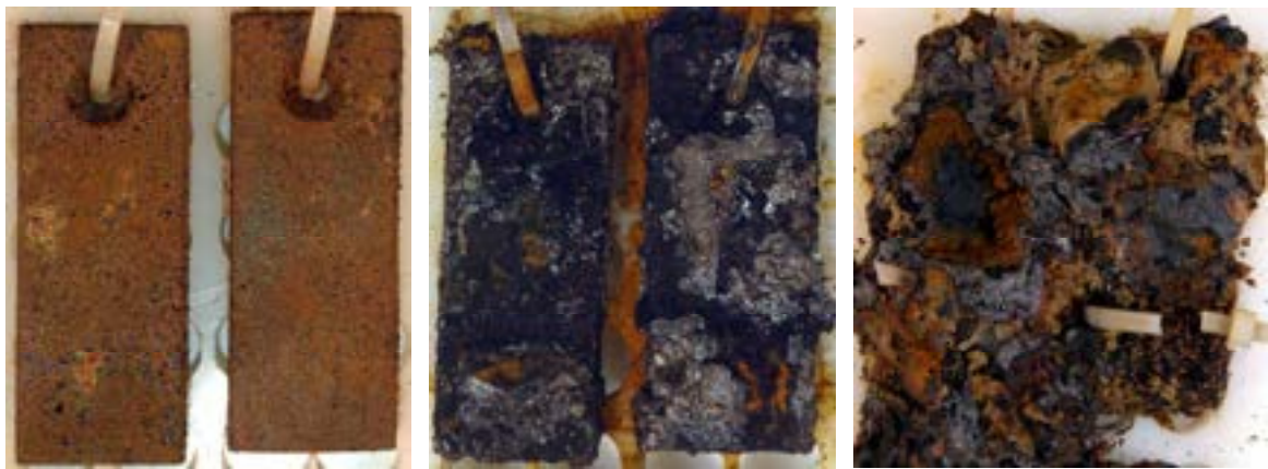
Figure 65. The cast iron coupons – just below sediment recovered in 2004 after 2 years of storage (left), in 2005 after 1 year of storage (mid) and in 2009 after 5 months of storage (right).
