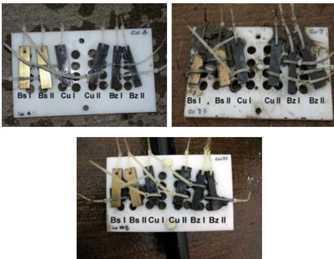
Figure 80. Copper alloy coupons – 50cm below sediment, immediately after recovery in 2004 after 1 year of exposure (top left), in 2005 after 2 years of exposure (top right) and in 2009 after 6 years of exposure (bottom).
