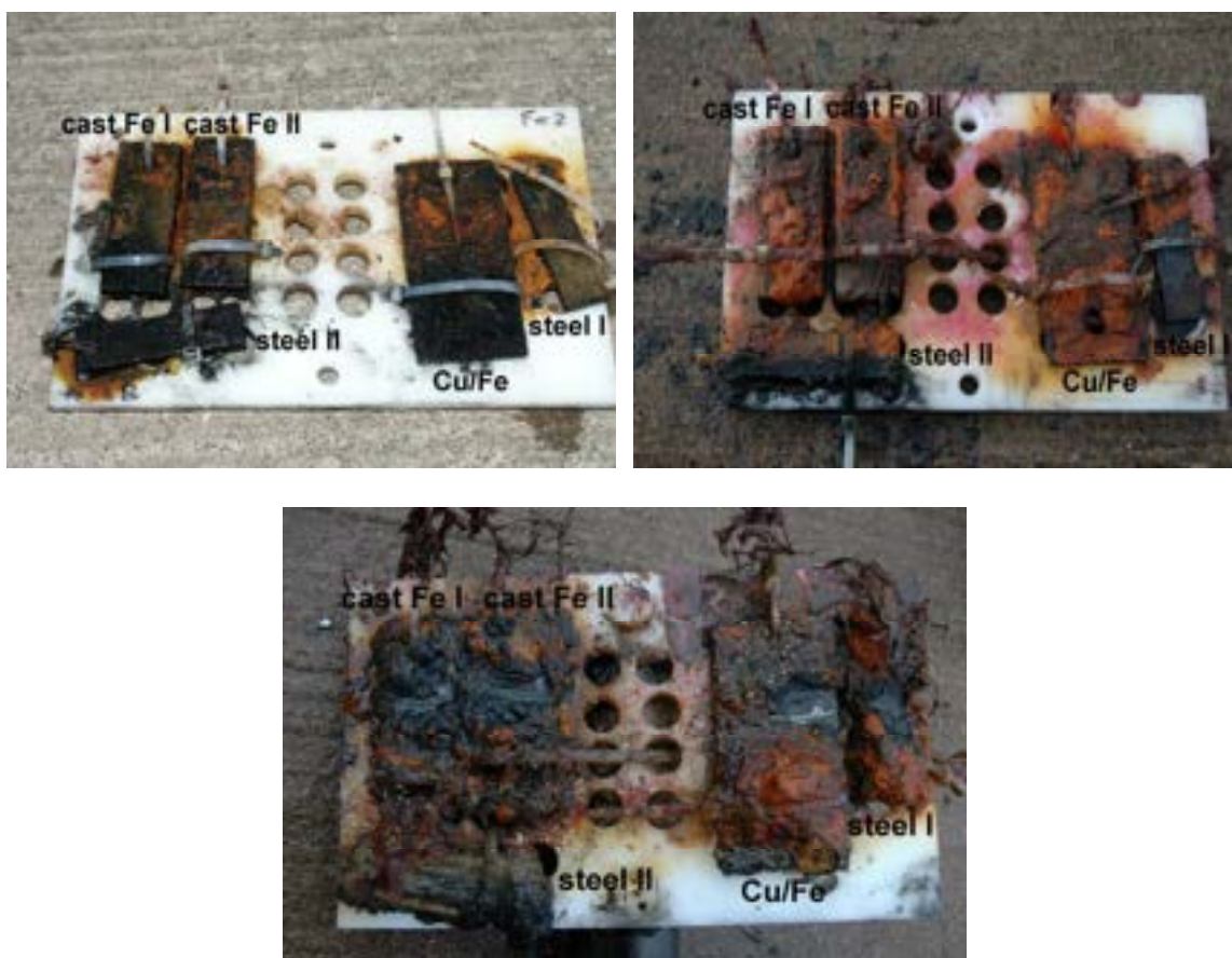
Figure 42. Ferrous alloy coupons – above sediment, immediately after recovery in 2004 after 1 year of exposure (top left), in 2005 after 2 years of exposure (top right) and in 2009 after 6 years of exposure (bottom).
