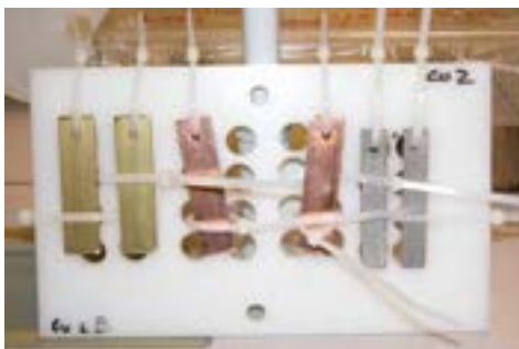
Figure 3. Completed metal alloy support plates: (left) copper alloy coupons; (right) ferrous alloy coupons.
