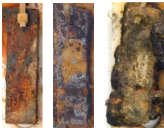
Figure 43. The mild steel coupons – above sediment recovered in 2004 after 2 years of storage (left), in 2005 after 1 year of storage (mid) and in 2009 after 5 months of storage (right).
