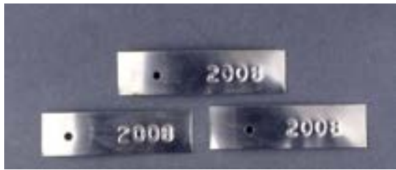
Figures 32 & 33. Steel Dymo labels. References and samples retrieved after seven years of in-situ exposures in the sediments.
