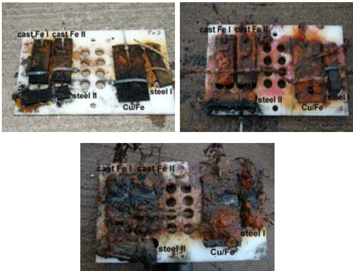
Figure 33. Ferrous alloy coupons – above sediment, immediately after recovery in 2004 after 1 year of exposure (top left), in 2005 after 2 years of exposure (top right) and in 2009 after 6 years of exposure (bottom).
