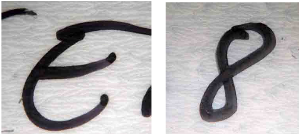
Figure 36 & 37. Permanent marker (Q) on PE bag. Reference and sample after seven years of exposure in situ.
