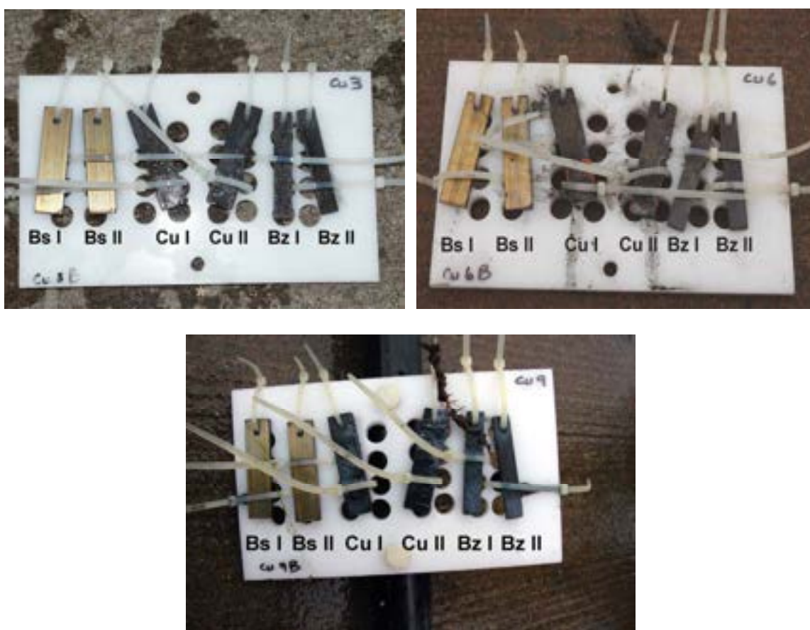
Figure 46. Copper alloy coupons – just below sediment, immediately after recovery in 2004 after 1 year of exposure (top left), in 2005 after 2 years of exposure (top right) and in 2009 after 6 years of exposure (bottom).
