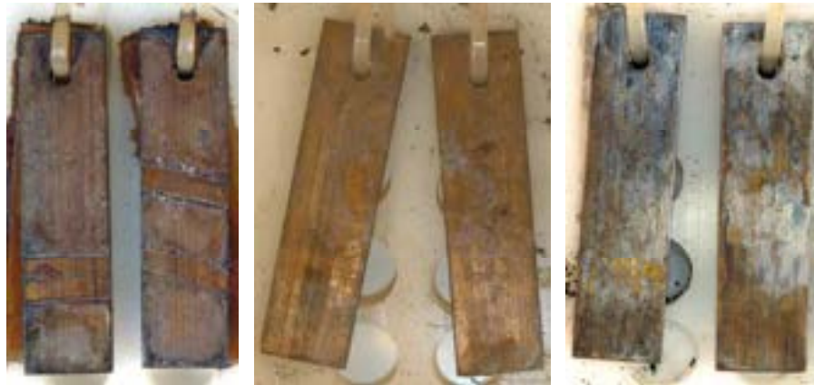
Figure 51. The brass coupons – just below sediment recovered in 2004 after 2 years of storage (left), in 2005 after 1 year of storage (mid) and in 2009 after 5 months of storage (right).
