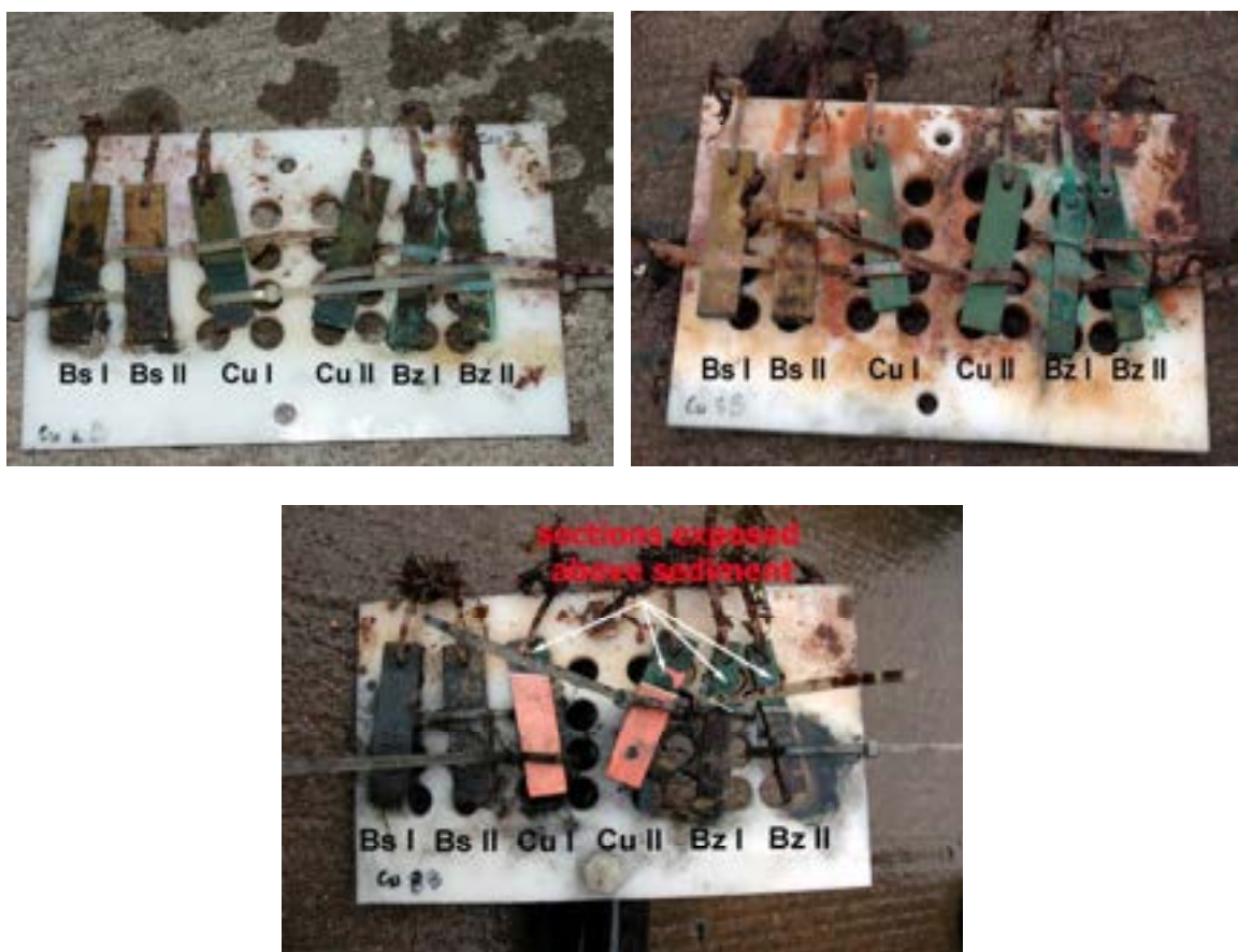
Figure 22. Copper alloy coupons – above sediment, immediately after recovery in 2004 after 1 year of exposure (top left), in 2005 after 2 years of exposure (top right) and in 2009 after 6 years of exposure (bottom).
