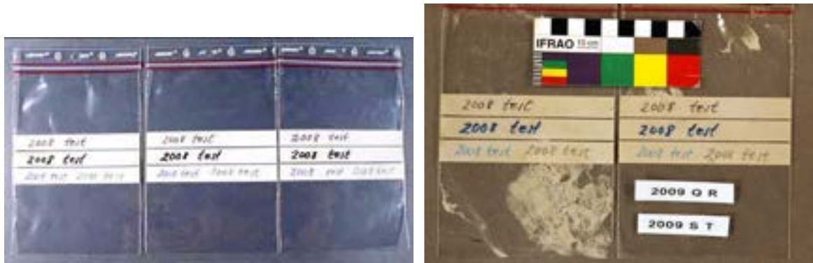
Figures 34 & 35. Written text on PE bags. References and samples retrieved after seven years exposure in-the sediments.
