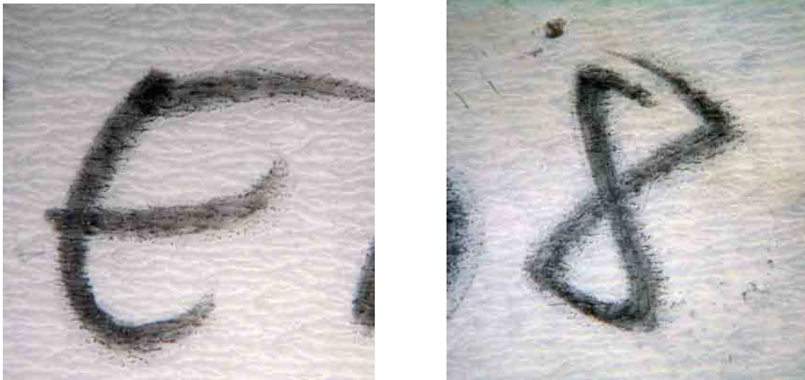
Figure 42 & 43. Pencil (T) on PE bag. Reference sample and sample after seven years of exposure in situ.
