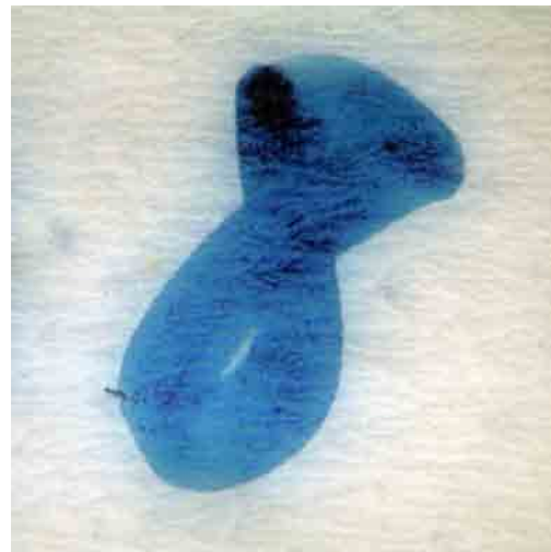
Figure 38 & 39. Permanent marker OH (R) on PE bag. Reference sample and sample after seven years of exposure in-situ in the sediments.
