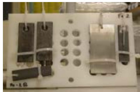
Figure 3. Completed metal alloy support plates: (left) copper alloy coupons; (right) ferrous alloy coupons.
