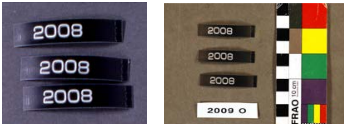
Figures 30 & 31. PVC Dymo labels. References and samples retrieved after seven years of in-situ exposures in the sediments.
