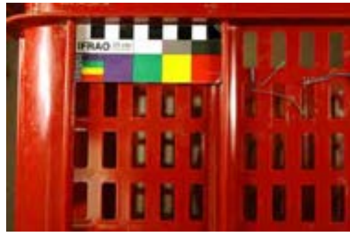
Figure 4 & 5. Close up of HDPE crate. Reference sample and sample after seven years of in-situ exposure in the sediments
