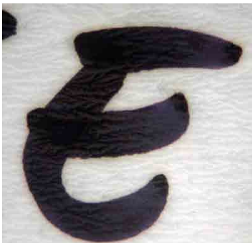
Figure 38 & 39. Permanent marker OH (R) on PE bag. Reference sample and sample after seven years of exposure in-situ in the sediments.
