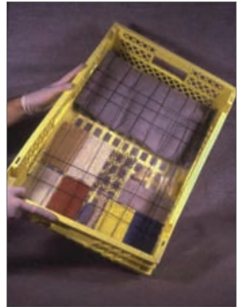
Figure 8. The non-wood organic materials sample unit containing one uncovered and one covered set of samples before burial in Marstrand harbour, September 2002 (photo Elizabeth Peacock, VM-NTNU).
