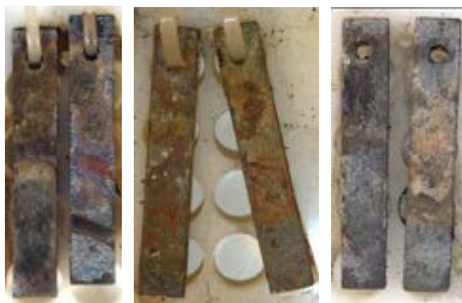
Figure 55. The bronze coupons – just below sediment recovered in 2004 after 2 years of storage (left), in 2005 after 1 year of storage (mid) and in 2009 after 5 months of storage (right).
