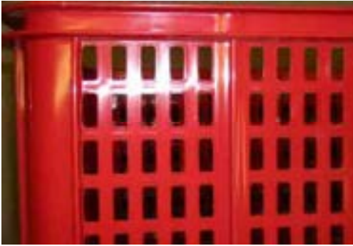
Figure 4 & 5. Close up of HDPE crate. Reference sample and sample after seven years of in-situ exposure in the sediments
