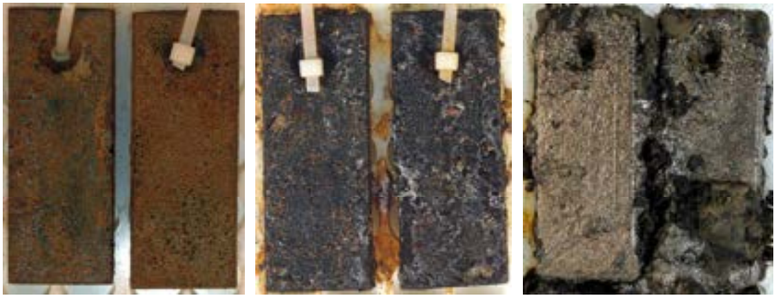
Figure 89. The cast iron coupons - 50cm below sediment recovered in 2004 after 2 years of storage (left), in 2005 after 1 year of storage (mid) and in 2009 after 5 months of storage (right).
