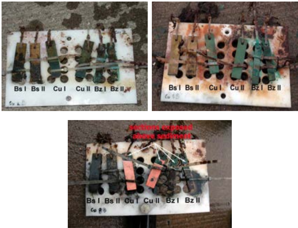
Figure 27. Copper alloy coupons – above sediment, immediately after recovery in 2004 after 1 year of exposure (top left), in 2005 after 2 years of exposure (top right) and in 2009 after 6 years of exposure (bottom).
