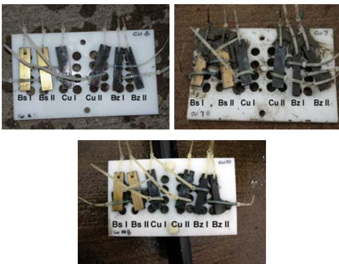
Figure 76. Copper alloy coupons – 50cm below sediment, immediately after recovery in 2004 after 1 year of exposure (top left), in 2005 after 2 years of exposure (top right) and in 2009 after 6 years of exposure (bottom).
