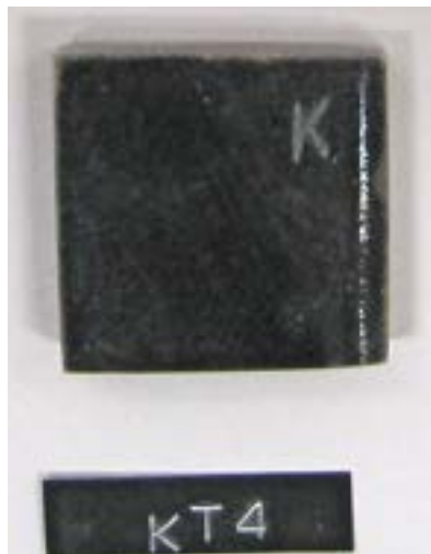
Figure 1b & c. Sample deposited in geotextile and retrieved after 7 years, in wet condition (b) and after drying (c)
