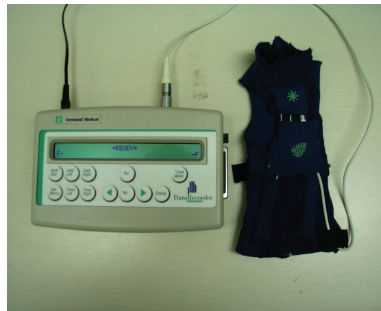
Figure 7 The instrumented glove used to measure wrist positions and movements
